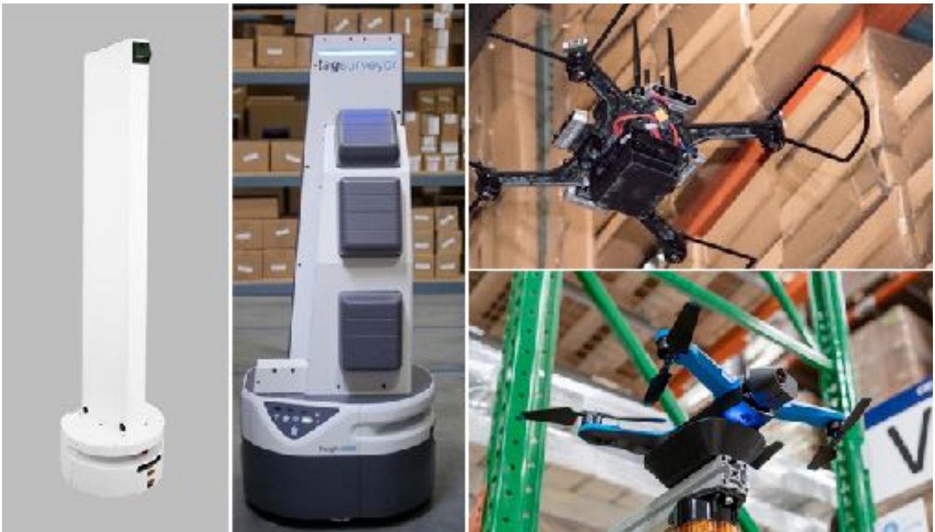
Figure 16 - Images of warehouse inventory counting robots/drones. (images courtesy of Keonn, Fetch Robotics, Ware Robotics and Corvus Robotics)
