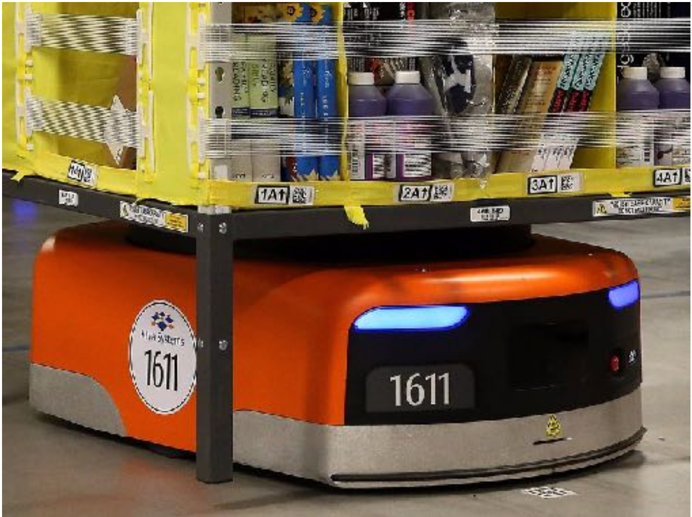
Figure 6 - This image illustrates a portable storage unit being moved with a Kiva Systems AMR. (Image courtesy of Amazon Robotics)
