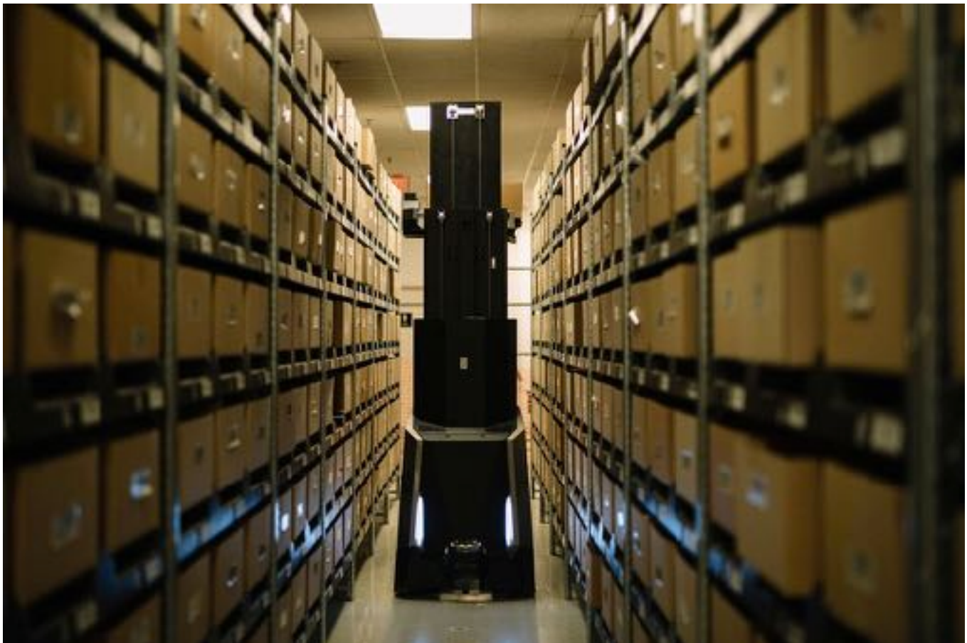
Figure 12 - Caja Robotics is an example of a bASRS solution that leverages existing warehouse shelving and bin storage to automate this workflow. (image courtesy of Caja Robotics)
