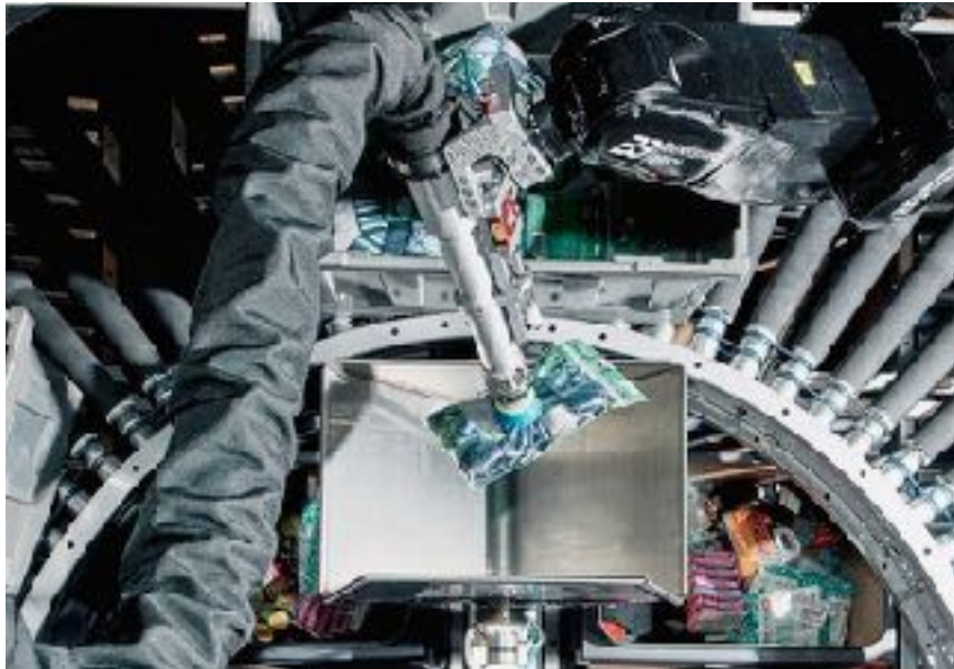
Figure 18 - Bin picking robots use vision and AI to identify items (Image courtesy of Berkshire Grey)
