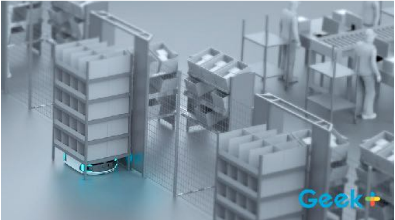
Figure 9 - Example of a typical picking station (image courtesy of Geek+ Robotics).
