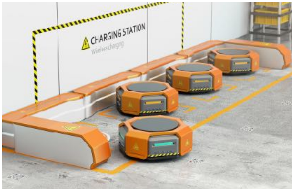
Figure 22 - Autonomous charging is a key feature that enables the AMR to keep its battery charged throughout its workday.
