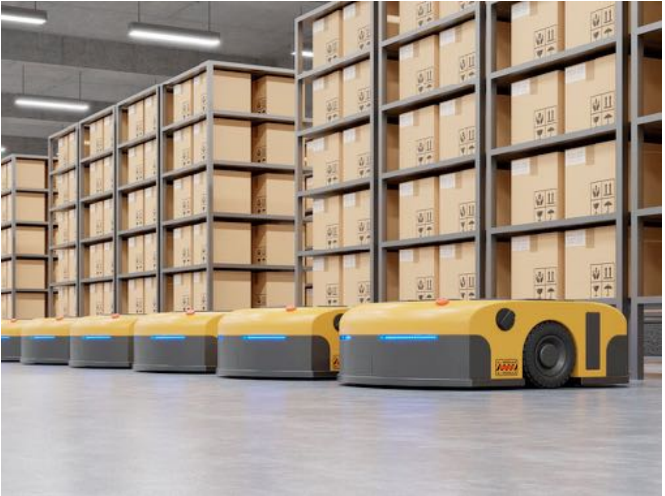
Figure 8 - Goods-to-person robot fleet with Associated product storage units. (istockphoto)
