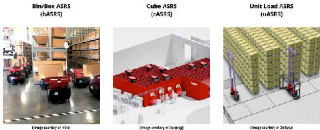
Figure 11 - The three categories of ASRS solutions. (l — bASRS, m — cASRS, r — uASRS)
